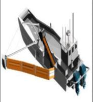
**Tactic purpose and description:** The purpose of this tactic is on-water recovery of oil in a protected or shallow water operating environment. To promote the ability for continuous recovery operations, the tactic assumes that recovered oil is off loaded to available on-water storage. See Storage Systems, "Shallow Water Barge" or "TBL Barge" for more information.
