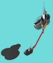
Tactic purpose and description: The purpose of this tactic is on-water recovery of oil in a protected or shallow water operating environment.
