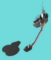
**Tactic purpose and description:** The purpose of this tactic is on-water recovery of oil in a protected or shallow water operating environment. Swath width is enhanced with 300' of boom and a workboat. To promote the ability for continuous recovery operations, the tactic assumes that recovered oil is off loaded to available on-water storage. See Storage Systems, "Shallow Water Barge" or "TBL Barge" for more information.
