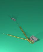
**Tactic purpose and description:** The purpose of this tactic is calm/protected/or fast water collection and storage. This tactic assumes the Buster will be deployed using two workboats capable of towing the unit. To promote the ability for continuous recovery operations, the tactic assumes that collected oil is off loaded to available on-water storage.
