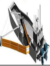
**Tactic purpose and description:** The purpose of this tactic is on-water recovery of oil in a protected or shallow water operating environment. To promote the ability for continuous recovery operations, the tactic assumes that recovered oil is off loaded to available on-water storage. See Storage Systems, "Shallow Water Barge" or "TBL Barge" for more information.
